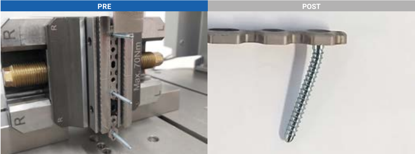
Locking Screw Angle Stability Results
