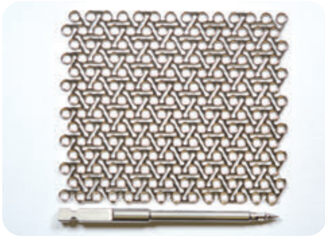
Close-up of mesh, showing pattern – including hole spacing measurement.
